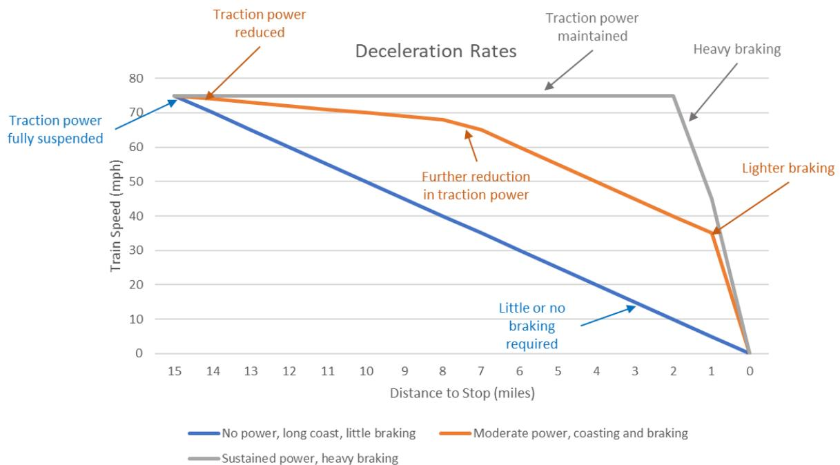
Even with regenerative braking, it is believed that approach number 3 will be the most energy efficient. The downside to this is the time taken to traverse the 15-mile section and the negative impact this may have on other services in the area. But it is for C-DAS to calculate the impact, make the most appropriate decision and deliver this to the driver.
